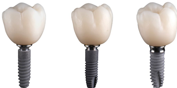
Fig. 3 Assembled specimens of the tested implant-abutment systems (from left to right): Ankylos C/X, Astra Tech EV, Xive S plus
